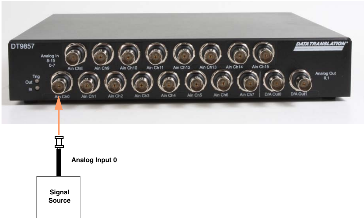
Figure 17: Connecting Analog Input Signals
